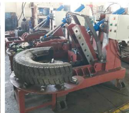
轮胎切断机 Whole Tire Cutter 将废轮胎切割成几个小块。 Cut the whole waste tires into small parts.
