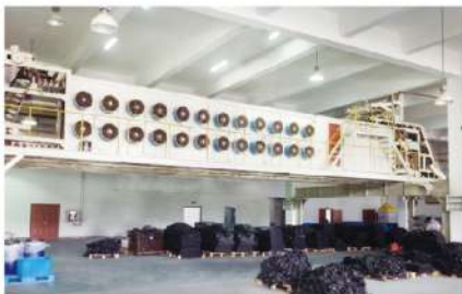
架空挂胶杆式 overhead hanging rods type
